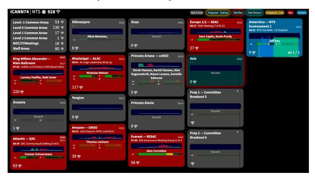
The NOC uses Zabbix to monitor all active equipment deployed into various areas of the venue. The tool enables the NOC to respond quickly to power outages, network problems, and equipment failures. The NOC is where the Meetings, Meetings Technical Services, and Security teams work together to ensure quick inter-departmental communications and coordination.
